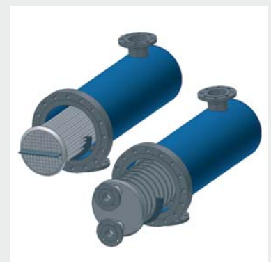
Figure 3: Illustration of tube bundle substitution by a stack of plate pairs.
